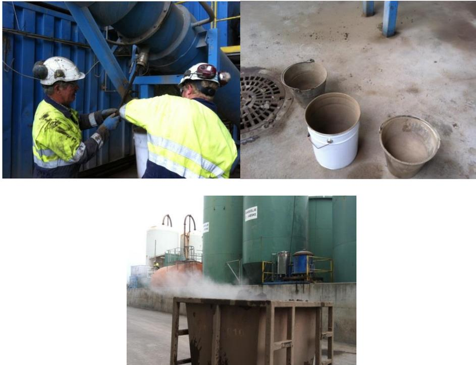
**Figure 14. Sampling treated cuttings (Out 17), cooling the sample and treated cuttings ready for disposal. Mongstad in August 2013.**
