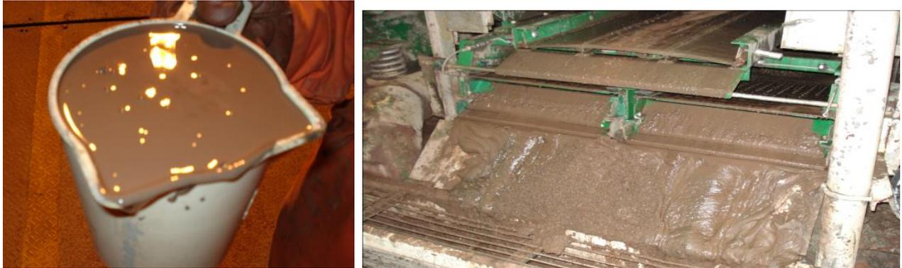
**Figure 8. OBM and OBM cuttings on the shaker. (Photo: Statoil)**
