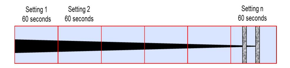
Ohmsett is 200 meter long (5-7 minutes of experimental time) for these towed experiments. Multiple experimental conditions (e.g. increased water velocity/rate) can be tested during one experiment.
