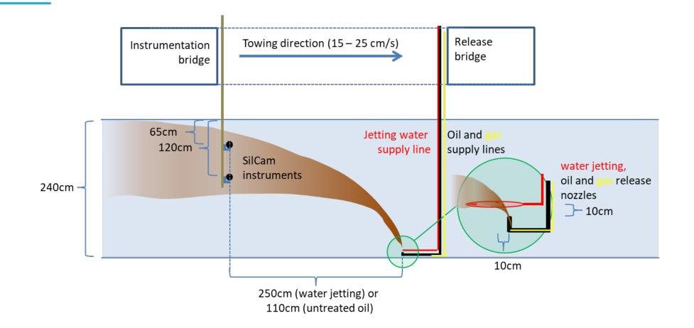
Arrangement for the combined releases of oil & gas and the water jetting
