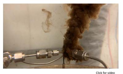
Smaller oil droplets and gas bubbles after water jetting
