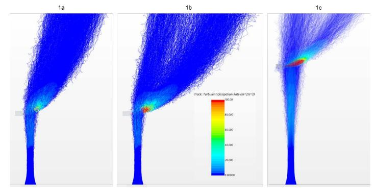
Release diameter: 0.50 m Release rate: 11 500 m<sup>3</sup>/day Gas to oil ratio: 50%
