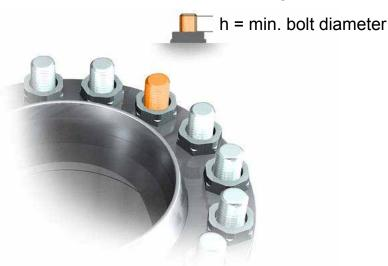
Lubricate the bolt's threads and the contact surface of the nut with an even layer of the given lubricant. Assemble the last nuts, so that LoaDisc is an underlay, between the nuts and flange on the side where the tool is installed.
