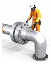
Immediately after the flanges are disassembled and cleaned, they should be inspected. Additional inspection personnel may be needed to perform an internal, visual inspection of pipes/equipment and inspect the ring track. If there is damage, this
