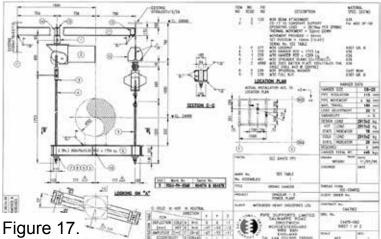
Example-drawing of a hanging arrangement with springs.
