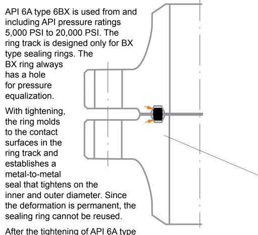
6BX flanges, the flange surfaces inside by the ring shall go completely or nearly completely together (almost no measurable gap).
