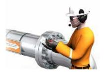
If it is necessary to use force beyond what is specified in "Alignment" to align the flange before normal tightening procedures can be started, this should be stated in the marking field in "Activity and inspection schedule" by the technician doing the work. This applies to all types of flange and clamp connections. The deviation should be recorded in the company's system for handling deviations.
