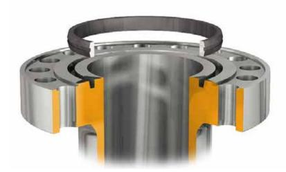
Metal-to-metal sealing ring deformation is checked. The sealing force between ring and ring track is not affected by dynamic forces since the tension in the bolts is taken up by the flange surface. This contributes to a static connection with nearly no flange movement, even when large dynamic forces are transmitted. This eliminates the need for post tightening of the bolts.
