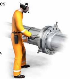
supervisor. Bolts and nuts should be checked for damage and the threads should be cleaned. Normally, galvanized bolts should not be reused.
