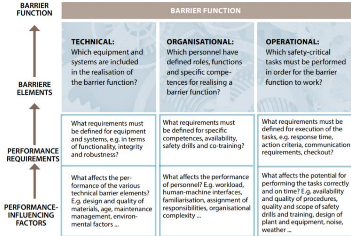
Figure 1-2 Relationship between barrier function, barrier elements, performance requirements and performance-influencing factors.
