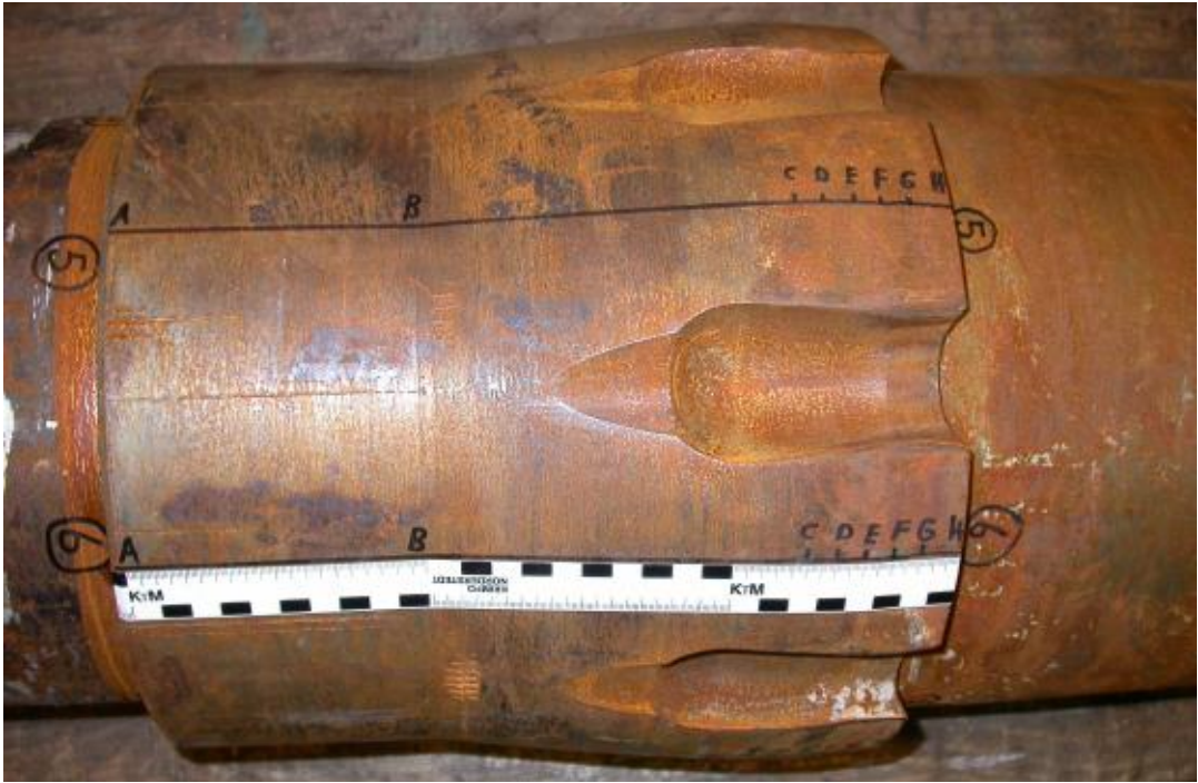
Figure 5 Deformed casing hanger after failure
