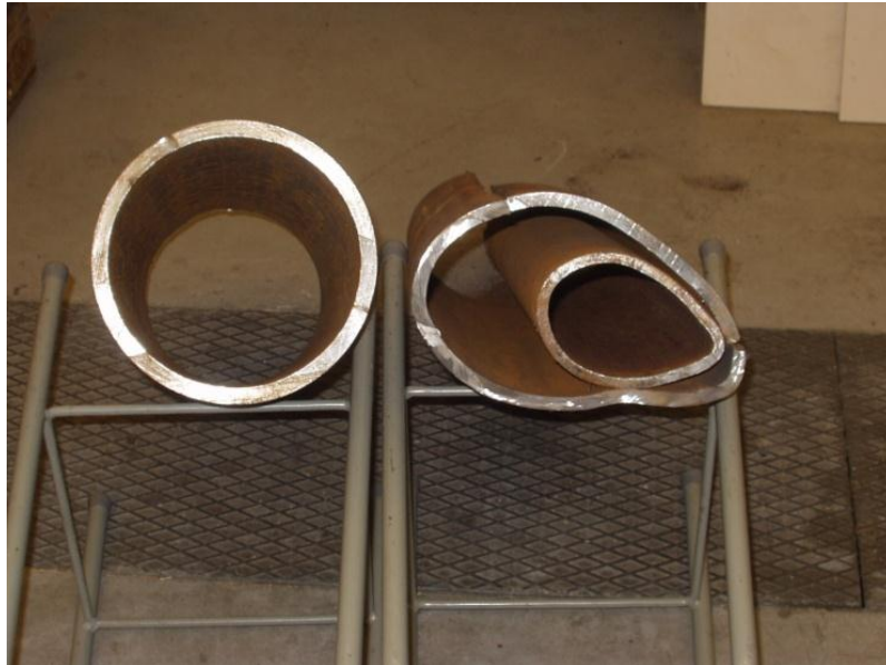
Figure 10 Failed production casing and production tubing
