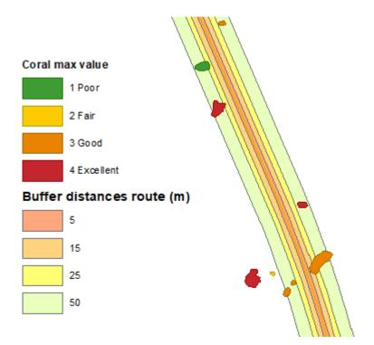
Figure 5-3 Example showing a planned pipeline and buffer distances from coral areas.
