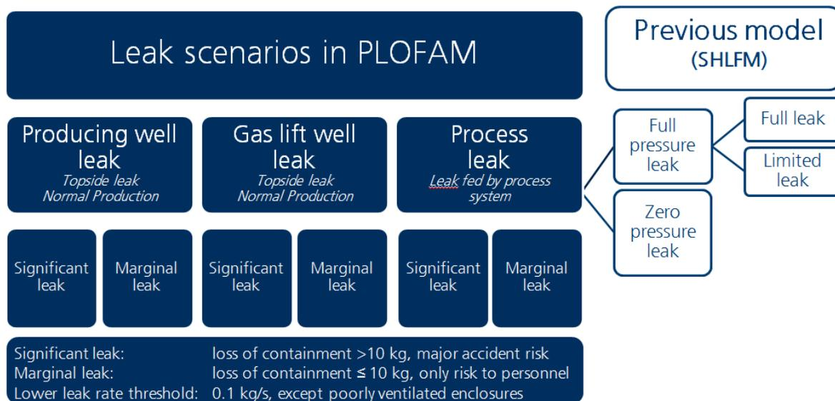
Figure 3.1 - Illustration and summary of the leak scenarios to be modelled in a QRA based on PLOFAM, together with the leak scenarios Full pressure leaks (Limited leaks and Full leaks) and Zero pressure leaks defined in the SHLFM Ref. /4/
