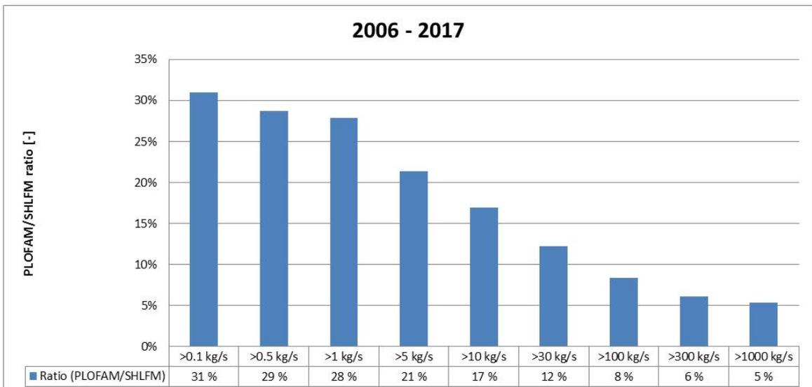
Figure 8.2 – Comparison of SHLFM and PLOFAM. The bars display the ratio per leak category for the total of gas and liquid leaks. For the SHLFM, only Full pressure leaks, i.e. Full leaks and Limited leaks are included. In PLOFAM, only significant leaks are included
