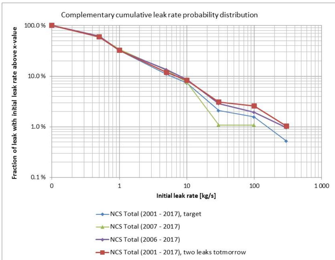
Figure 9.2 – Relative leak rate distributions for the periods 2001 – 2017 (target for model), 2006 – 2017, 2007 – 2017, and 2001 – 2017 including two leaks >100 kg/s where one leak is larger than 300kg/s potentially occurring tomorrow
