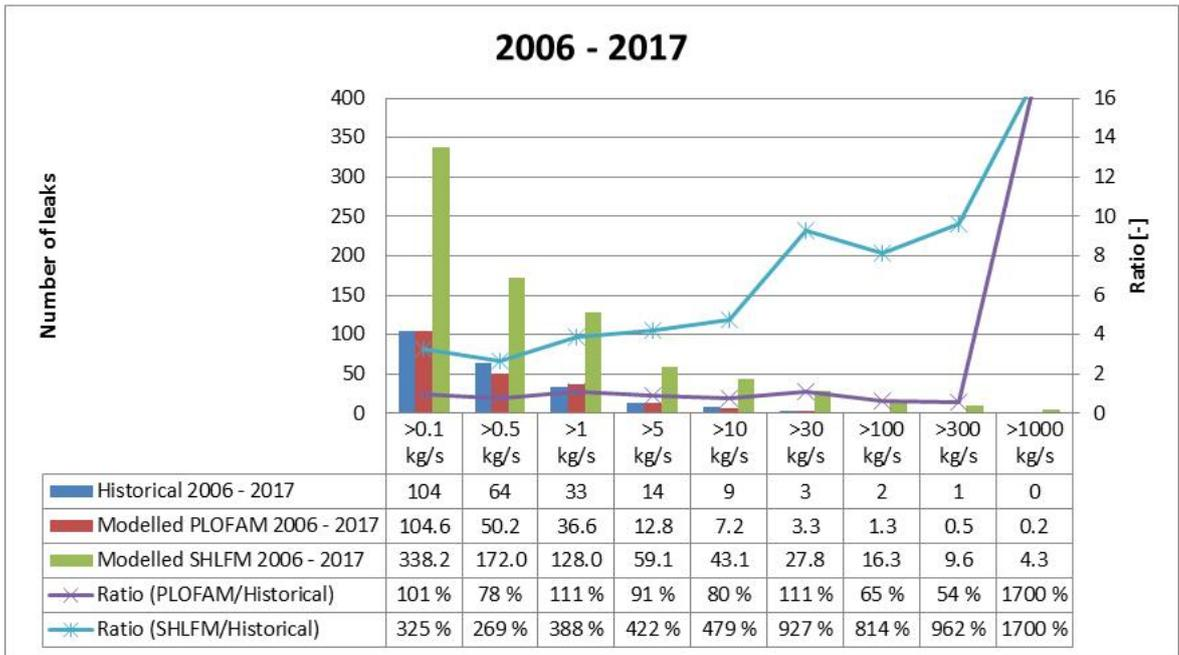
Figure 8.1 – Comparison of SHLFM and PLOFAM. The frequency is the sum of frequency for gas and liquid leaks. For the SHLFM model, only Full pressure leaks and Limited leaks are included. In PLOFAM, only significant leaks are included. Note that the ratio for leaks >1000 kg/s is infinite but plotted as 1700% to illustrate in the figure that the value is high
