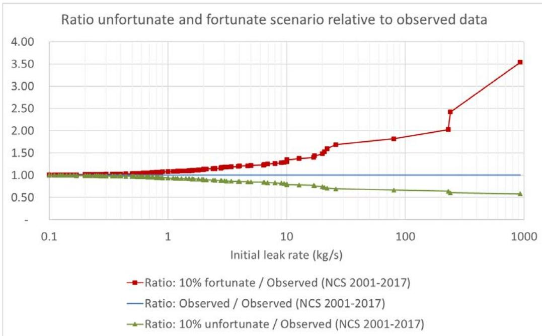
Figure 9.1 – Ratio unfortunate and fortunate scenario (10% percentiles used) with respect to observed data (NCS 2001-2017) versus initial leak rate. These ratios are derived directly from the relative leak rate distributions shown in TN-6
