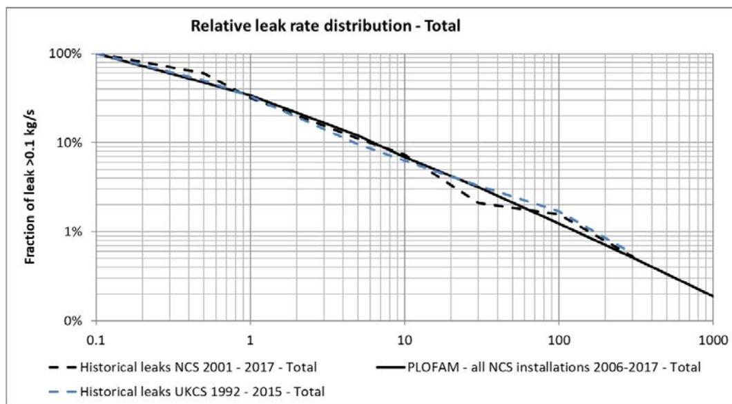
Figure 6.2 – Overall significant leaks: complementary cumulative relative leak rate distribution for all installations operating at NCS in the period 2006-2017
