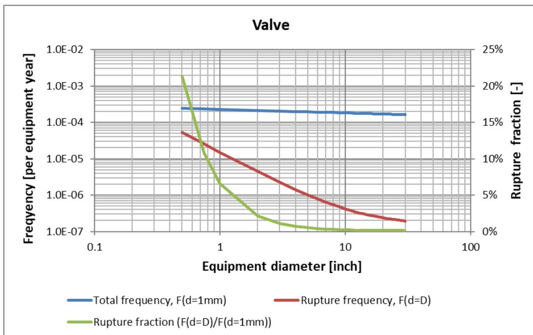
Figure 6.1 – Total frequency, rupture fraction (full bore hole fraction) and rupture frequency for valve
