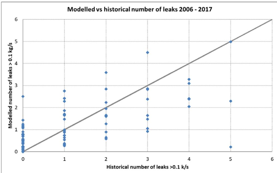
Figure 6.4 – Overall significant leaks: observed number of leaks vs. predicted number of leaks for all installations operating at NCS in the period 2006-2017. Datapoints below the grey line indicate underprediction. Datapoints above the grey line indicate overprediction
