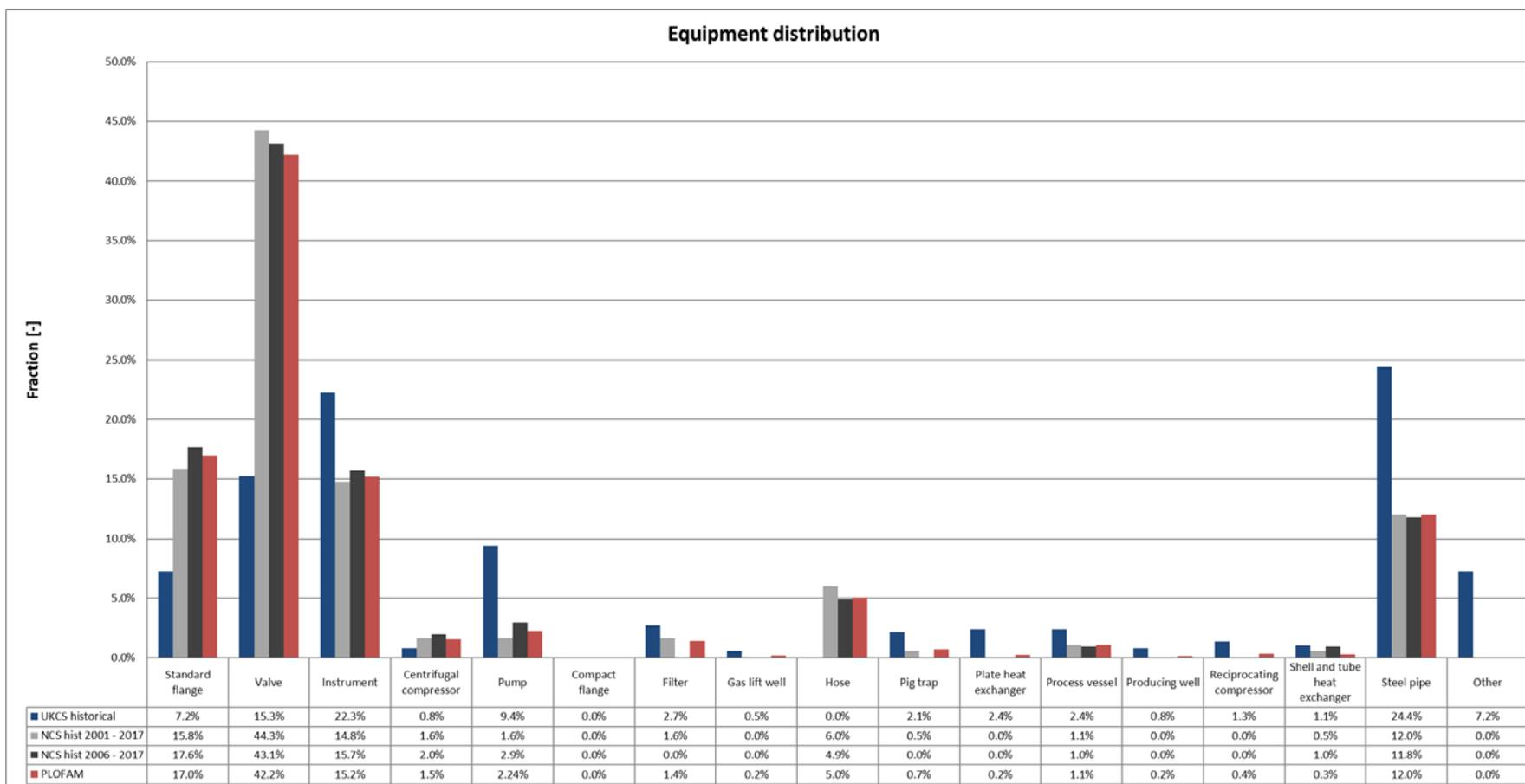
Figure 6.6 – Historical (both for NCS and UKCS) and modelled equipment type distribution for Significant leaks. Both the historical equipment type distribution for the period 2001 – 2017 and 2006 – 2017 are given. The modelled result is achieved by applying PLOFAM to all installations at NCS being in operation in the period 2006 – 2017
