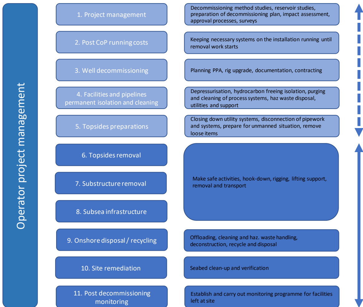
Figure 4-1. Decommissioning phases in the context of the IA's scope (solid arrow: base case, dotted arrow: scope to be addressed but not assessed in detail unless sufficient information is available). Source: Norwegian Oil and Gas decommissioning WBS handbook [13].
