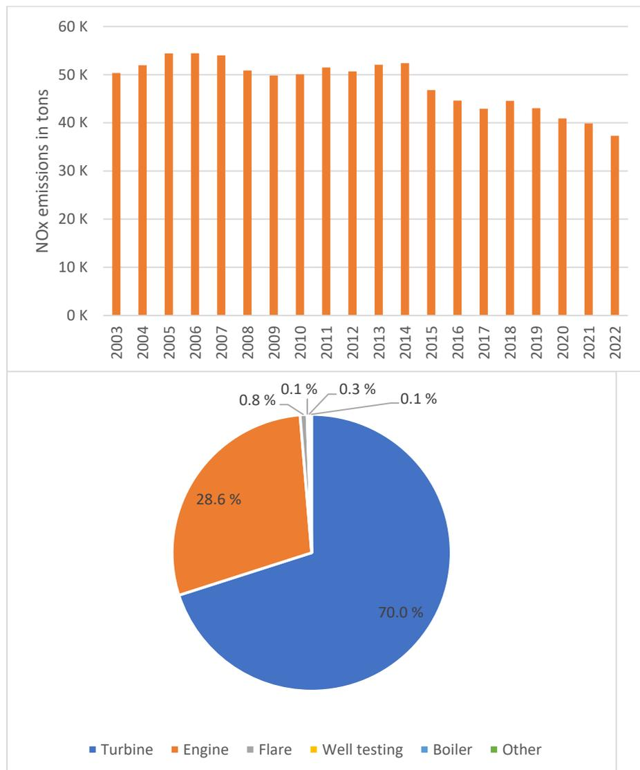
Fig 28: Historical development of total NOx emissions (in tons) and breakdown by source
