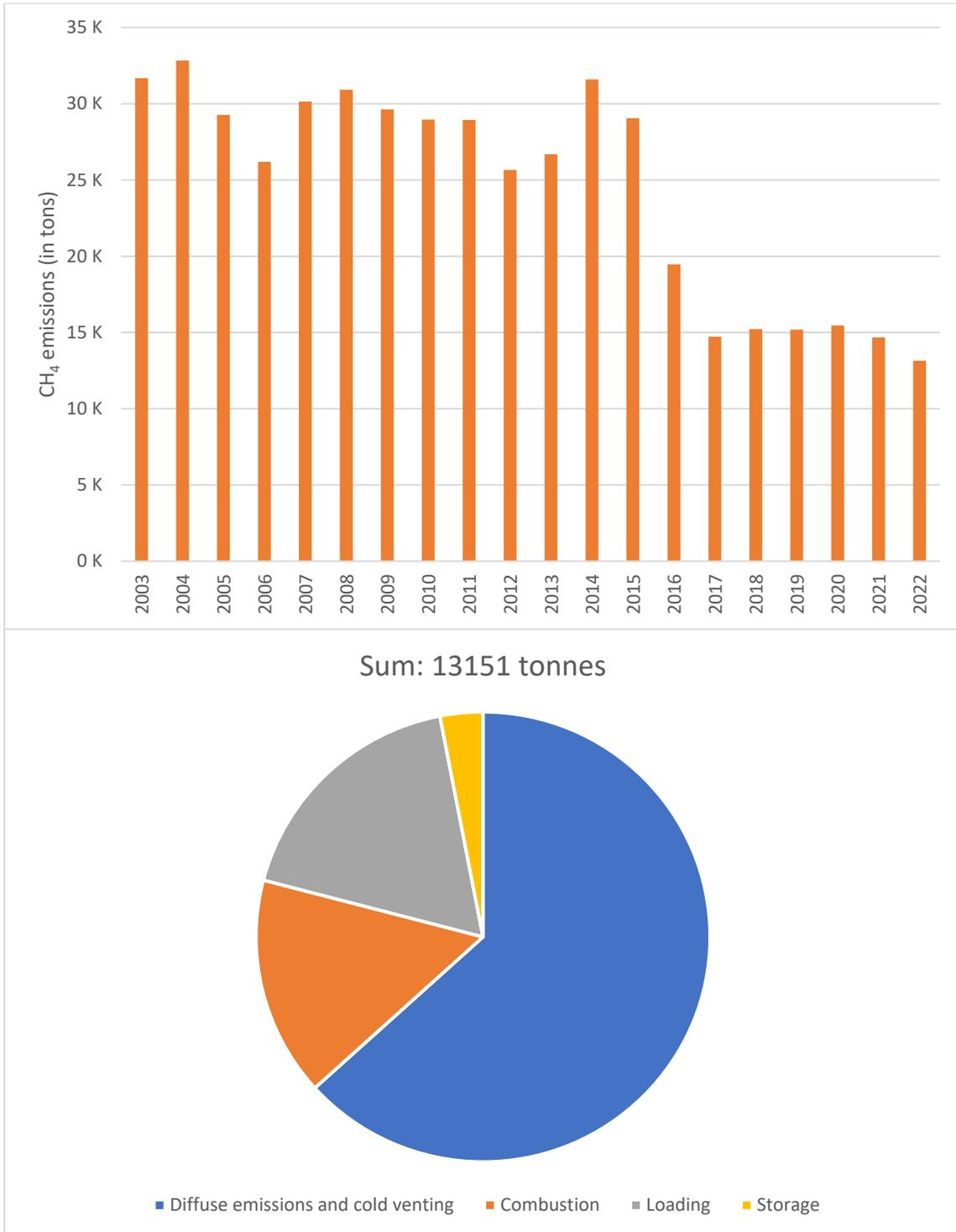
Fig. 26: Historical development of total emissions of CH<sub>4</sub> (in tons) and distribution by source
