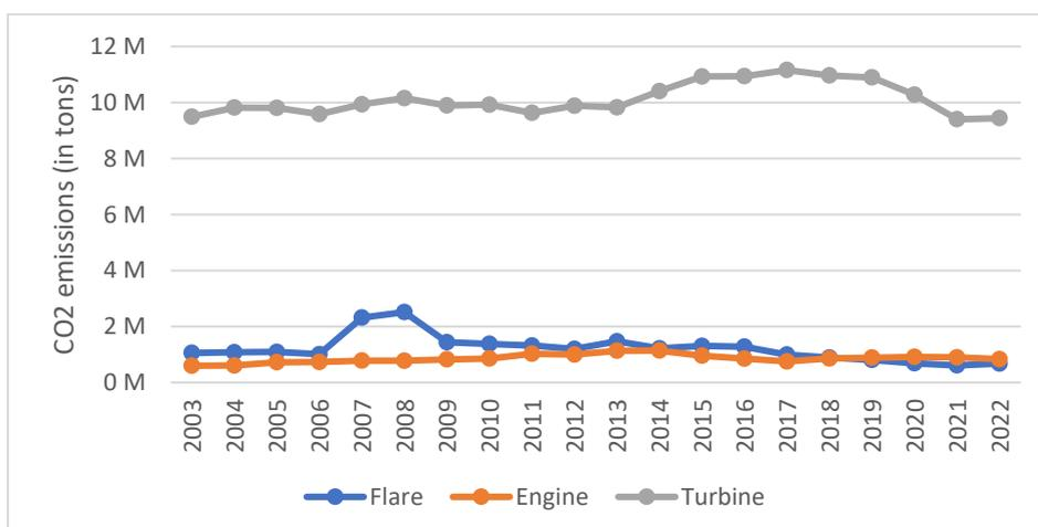
Fig. 24: Historical development of direct CO<sub>2</sub> emissions (in tons) from the three primary sources
