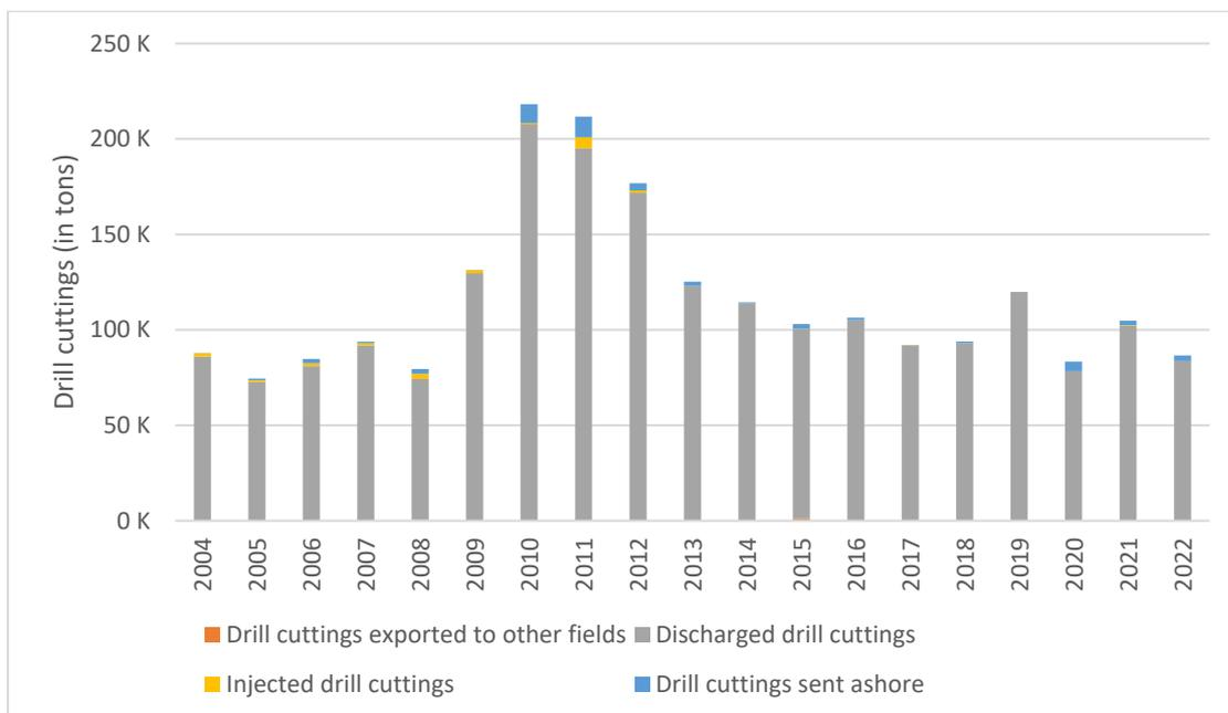
Fig. 6: Disposal of drill cuttings from wells drilled using water-based drilling fluids
