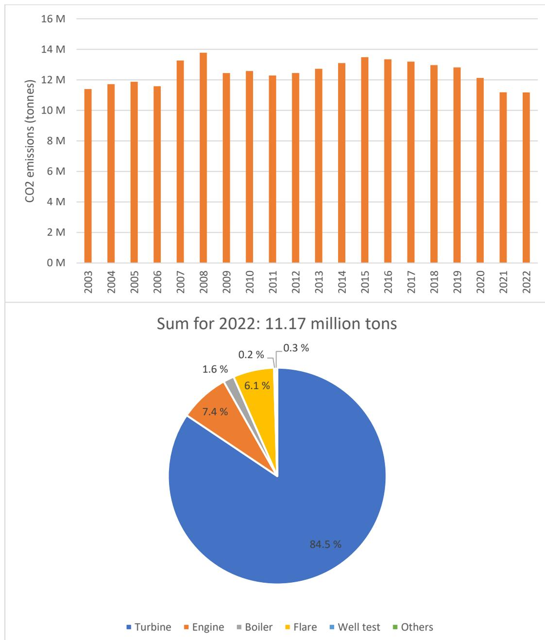
Fig. 22: Historical development of direct CO<sub>2</sub> emissions (millions of tons and distribution according to source)
