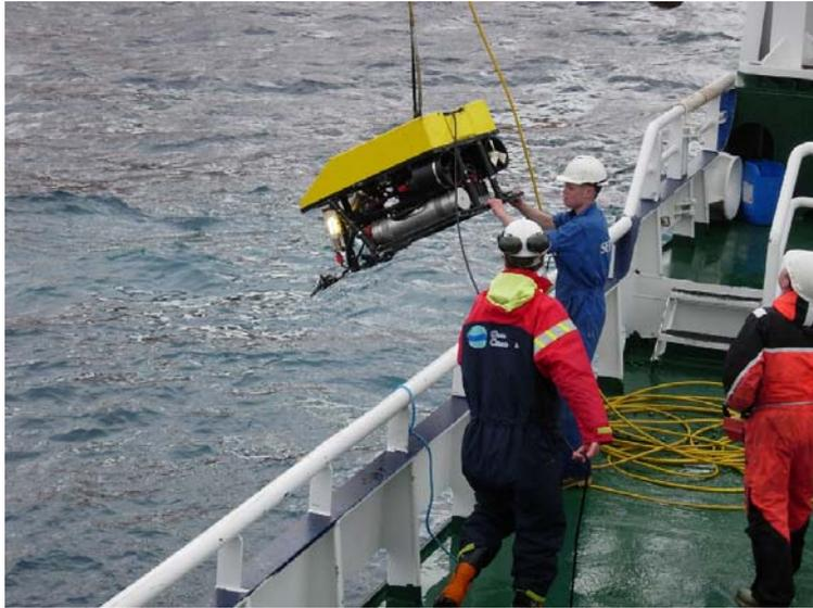
Figure 7. Retrieval of cage at mussel station 800 was facilitated by ROV due to damaged surface floats.
