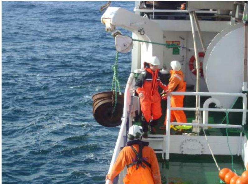
Figure 4. Launching of bottom mooring weight
