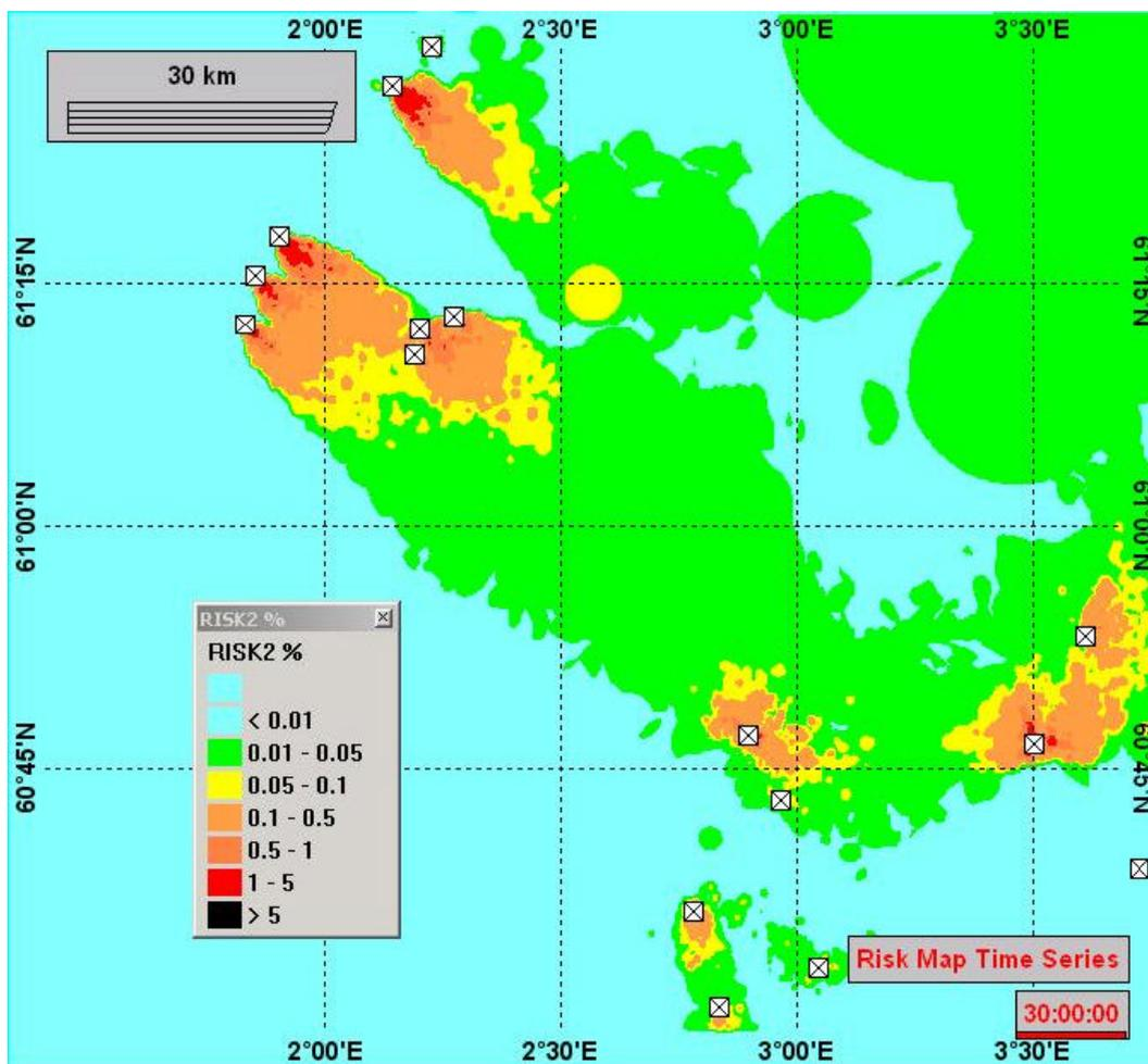
Figure 6.12 Simulation of the Tampen area NOEC 40 ng/l . Areas with PEC/NOEC>1,0 are shown in black.
