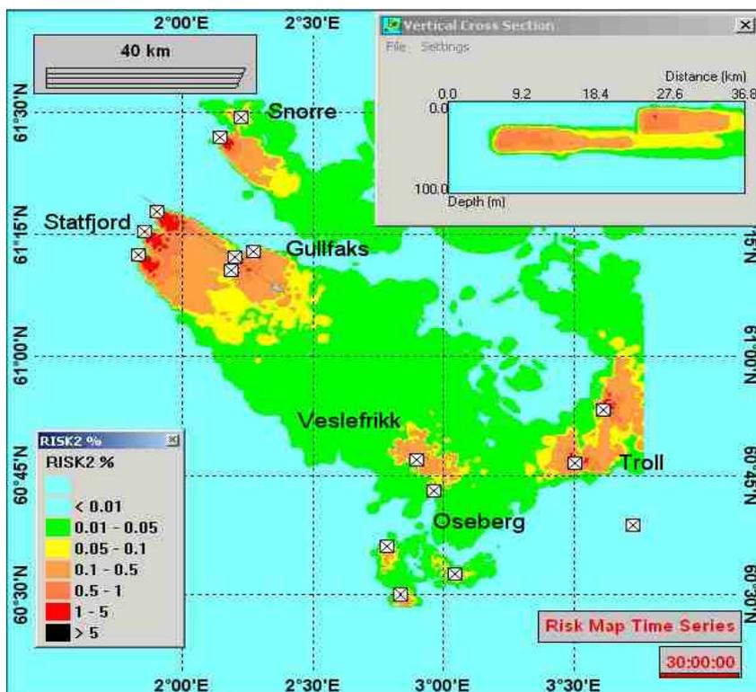
Figure 6.1 Simulation of the Tampen area, NOEC 40 ng/l . Areas with PEC/NOEC>1,0 are shown in black.
