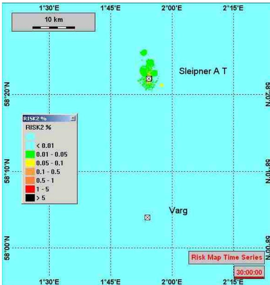
Figure 6.10 PEC/NOEC map of Sleipner and Varg showing the maximum risk area for the simulation.
