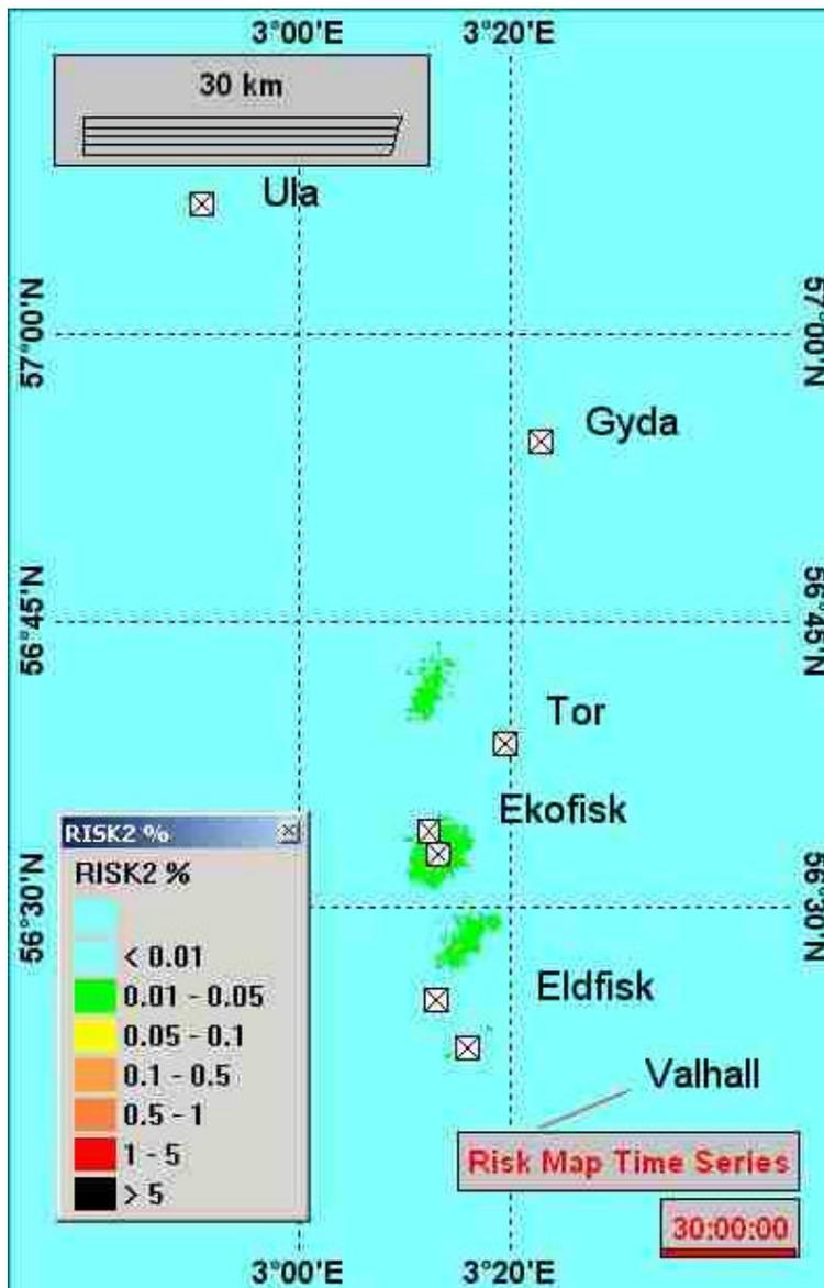
Figure 6.11 PEC/NOEC map for Ekofisk showing the maximum risk area for the simulation.
