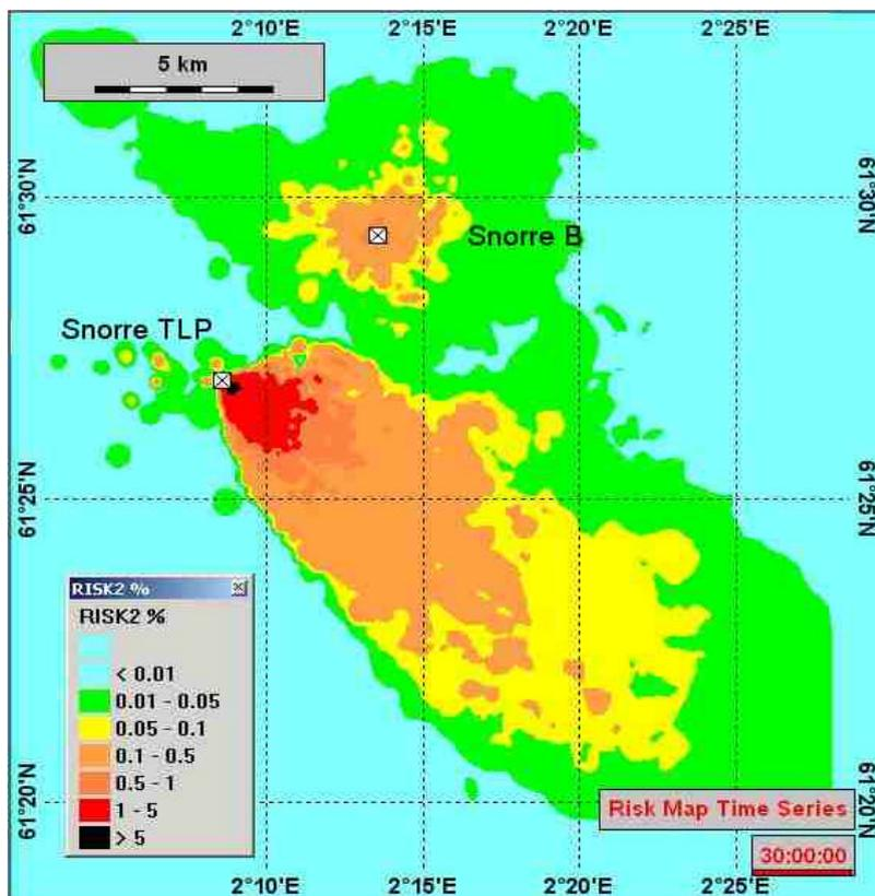
Figure 6.6 Simulation of the Sub-region Snorre, NOEC 40 ng/l.
