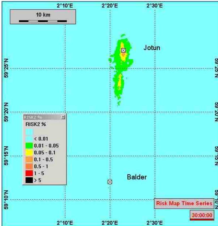
Figure 6.9 PEC/NOEC map of Jotun and Balder showing the maximum risk area for the simulation.
