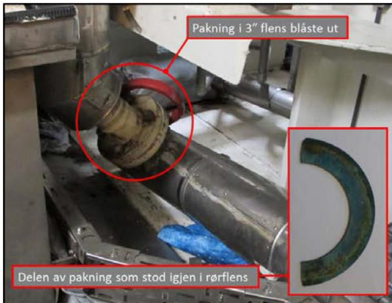
Figure: Red ring indicates where the gasket in the three-inch flange blew out.
