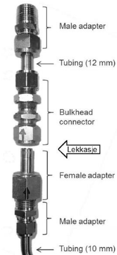
Figure 3: Erroneously installed fittings.
