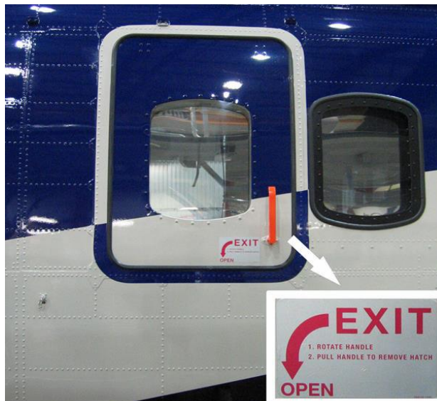
Fig. cabin emergency exit
