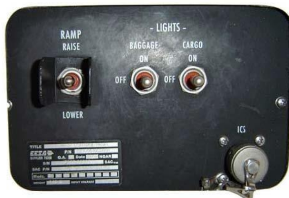
RAMP CONTROL PANEL
