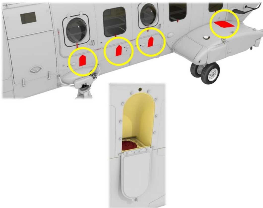
Fig. 6 Gravity refuelling point
