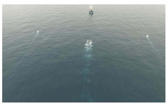
P-cable with 18 x 100m x 12.5m streamer spread and dual source (Wisting, 2016)
