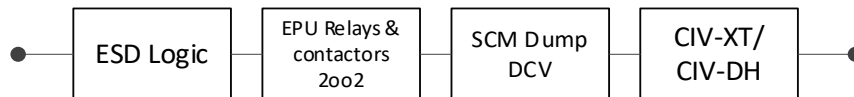
Figure A.13.8 RBD for the SIF "Isolation of chemical injection line in one subsea well".
