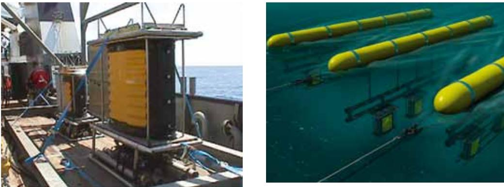
Figure 26 – marine vibrator (credit: Petroleum Geo-Services)
