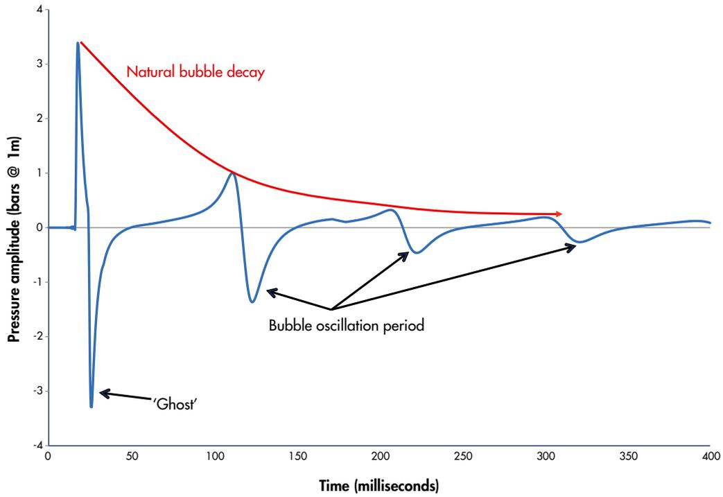
Figure 18a – Source signature of a single airgun (credit: Polarcus)
