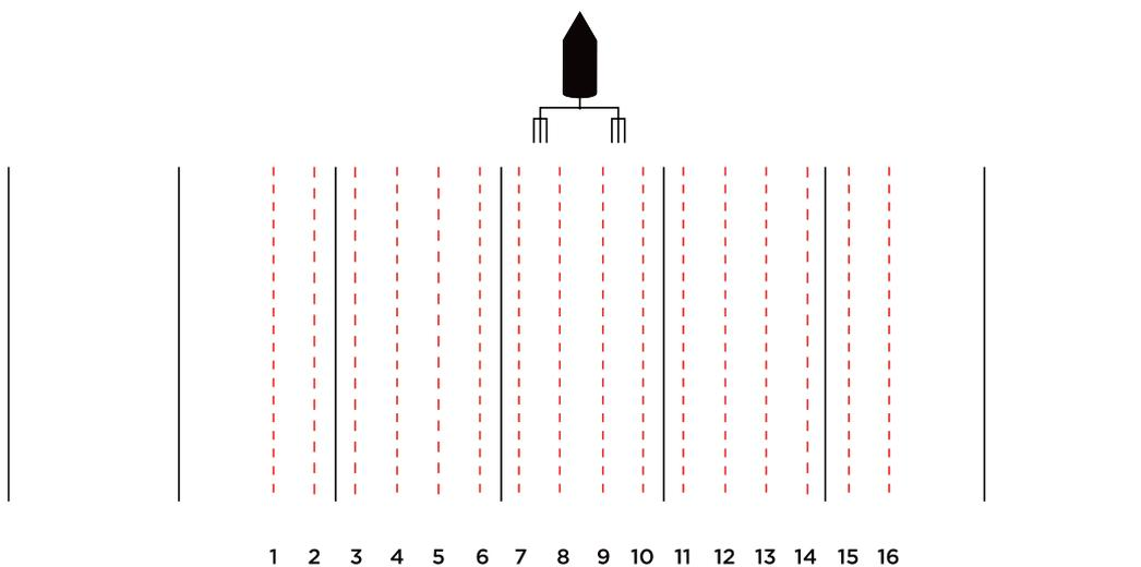
Figure 9 – schematic diagram of an 8-streamer, dual-source operation (credit: Chris Walker)
