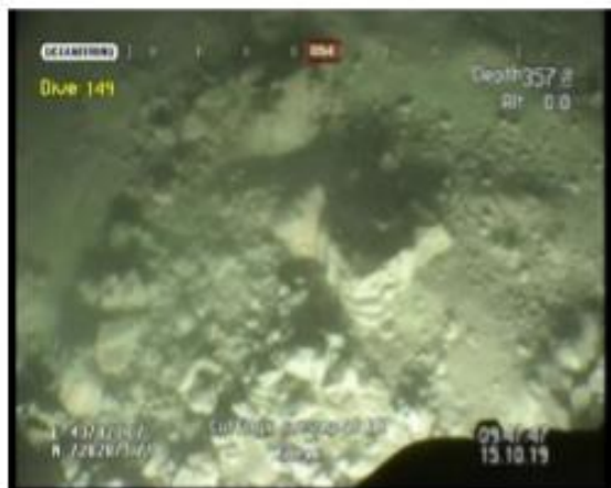
Figure 4-29: Cuttings 21 meters from wellbore.
