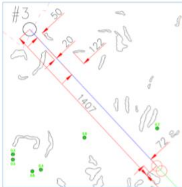
Figure 10: Overview over Anchor line #3 including bathymetry showing areas for potential coral presence
