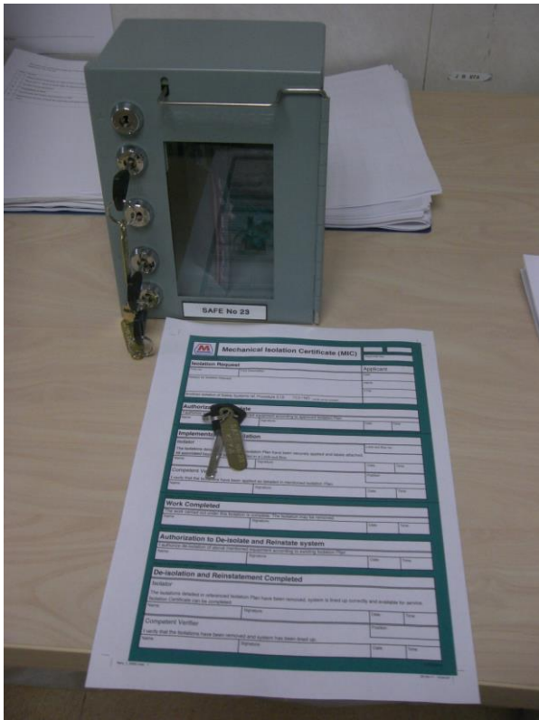
Figure 13 Example of a locking system (right) and lock-out box (left)
