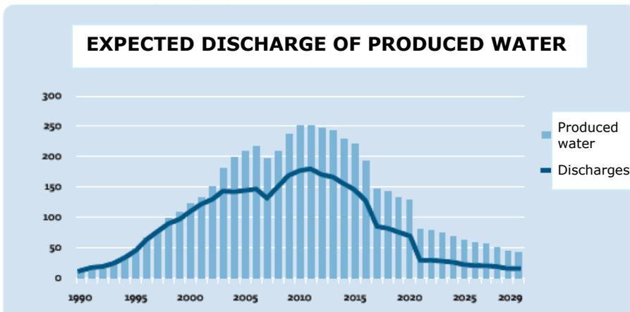
The graph shows how the volumes and discharges of produced water have developed on the Norwegian Shelf, and how the trend is expected to continue. The discharges are considerably lower than the total volume, thanks to use of reinjection.
