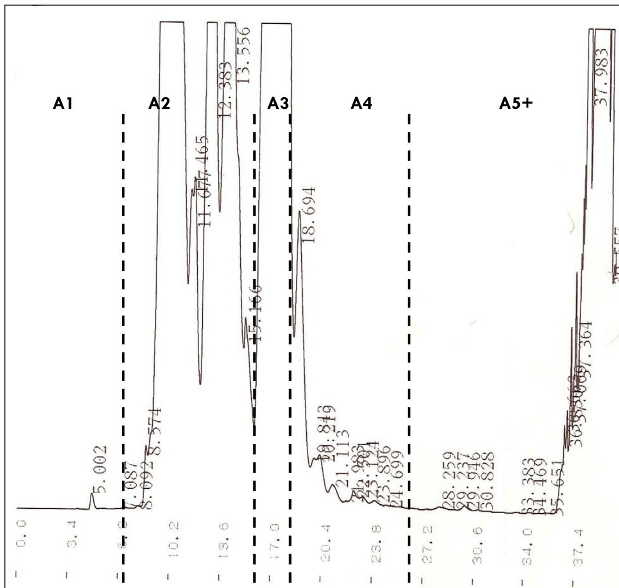
Figure 4. Ring-size separation (A1: 1-ring aromatics, A2: 2-ring aromatics, A3: 3-ring aromatics, A4: 4-ring aromatics, A5+: 5-ring aromatics and higher molecular aromatics) by normal phase HPLC.
