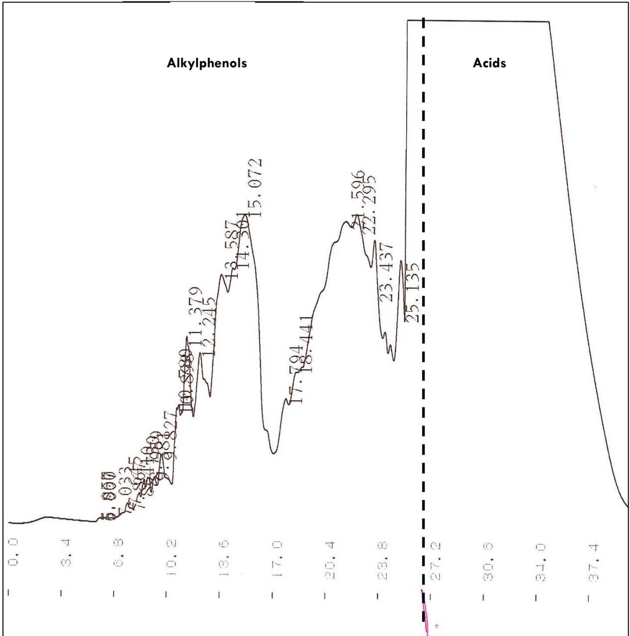
Figure 5. Separation of alkylphenols from acids by normal phase HPLC
