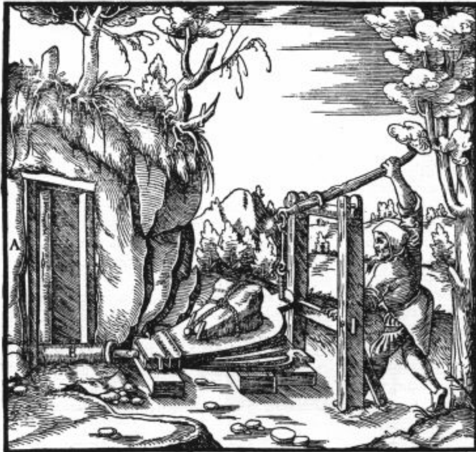
A—TUNNEL. B—PIPE. C—NOZZLE OF DOUBLE BELLOWS.
