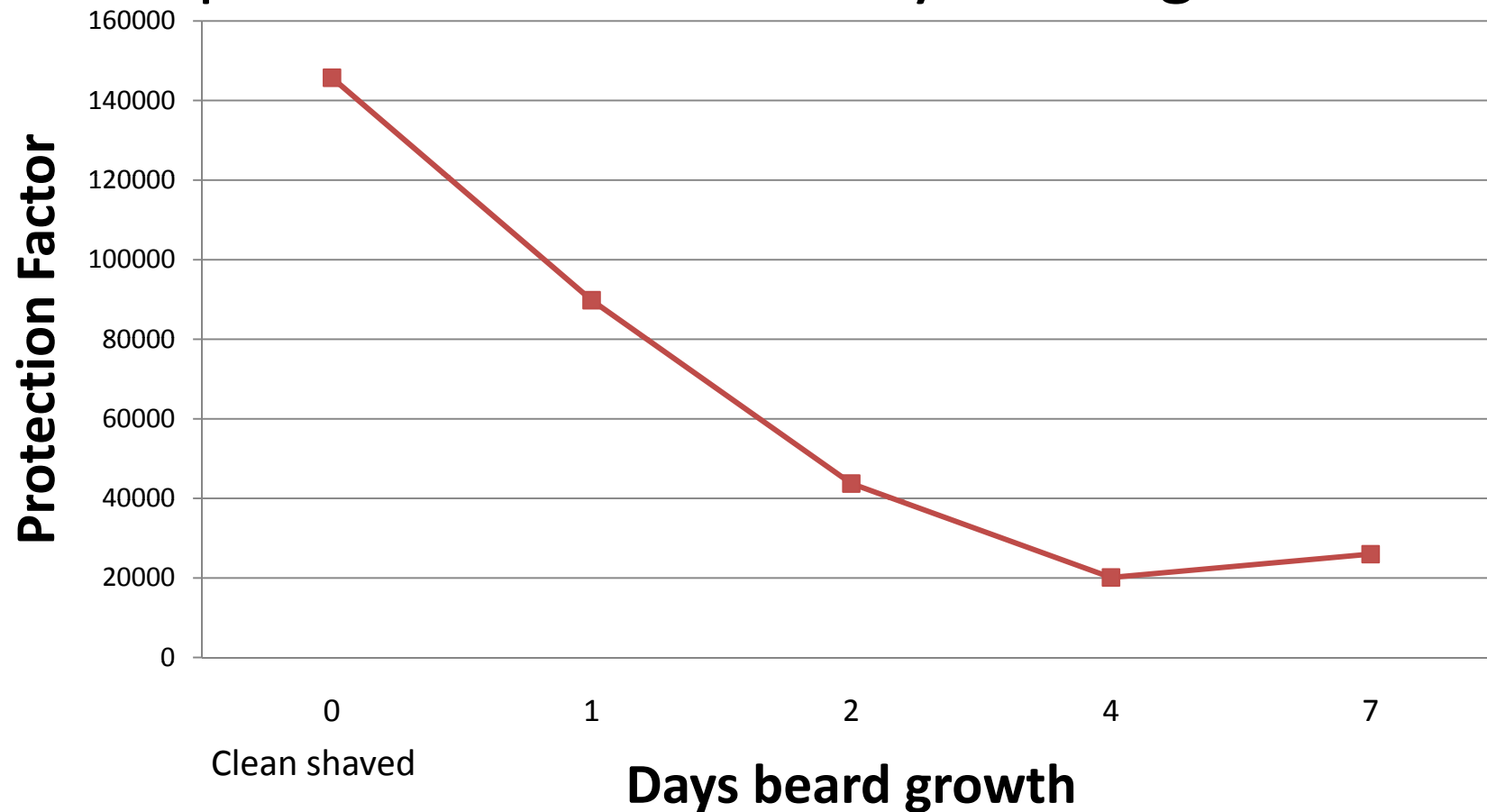
Figure 6. Protection factor for one test person with different beard length, using a negative pressure respirator.
