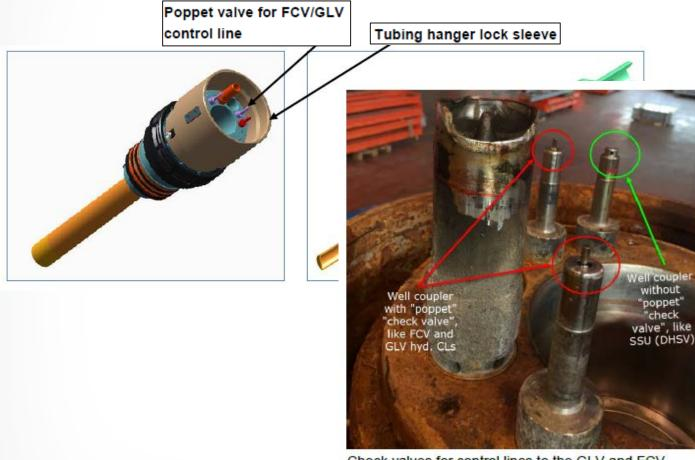
Check valves for control lines to the GLV and FCV circled in red Seen from the top of the tubing hanger
