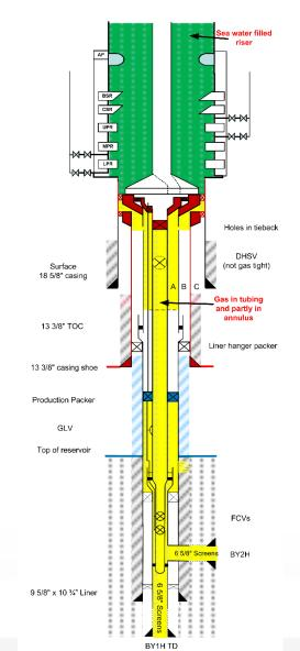
Primary barrier (GLV and FCV's) failed. Few hours later, when landing Tubing Hanger Secondary Retrieval Tool (THSRT) and preparing to pull Tubing Hanger, the well is already displaced to gas.
