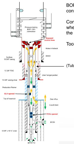
BOP/WH connector test. Exposed control lines for gas-lift valve (GLV) and flow control valves (FCV).
