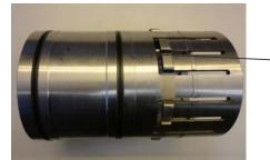
O-rings on sliding sleeve were leaking
