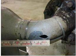
Figure 6 Hole eroded in the bend. Photo: Statoil.
