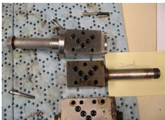
Picture 3, new and old hydraulic control valves
