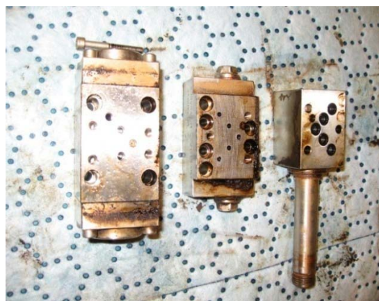
Picture 2, hydraulic control block disassembled
