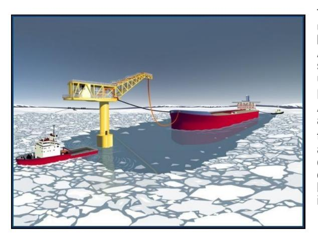
The export tanker moors up to the TLU and an ice breaker tug fitted with the Aquamaster propulsion system positions itself updrift from the TLU. By spreading the Aquamasters at approximately 80 deg. the tug maintains position and the propeller wash creates a wide swath of open water, the technique has been used and proven in Vityaz operations.
