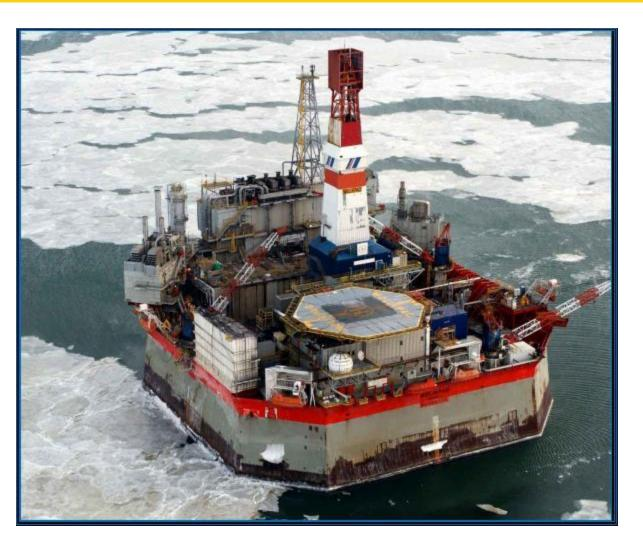
Converted drilling rig first used in the Canadian Arctic.
