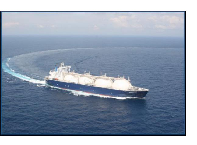
The 145 000 m<sup>3</sup> LNG carrier Grand Elena shown here is an Ice Class 1C vessel purpose built for the project. It is one of 5 purpose built vessels for the project.
