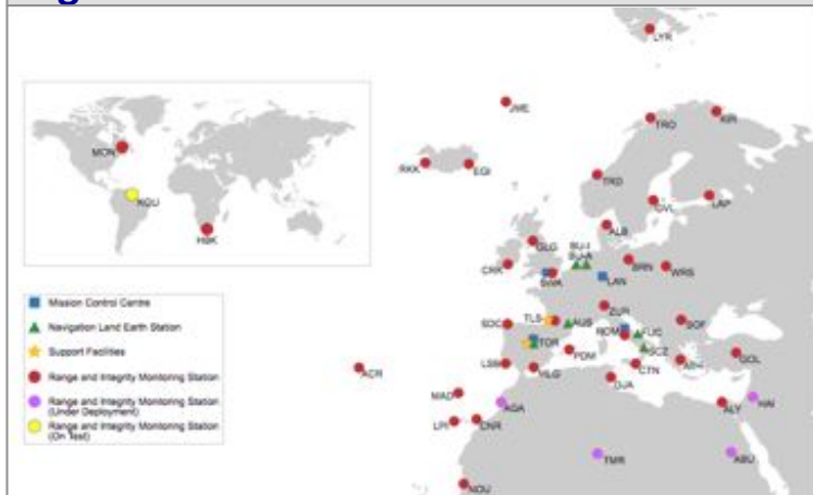
RIMS – ranging and integrity monitoring station
