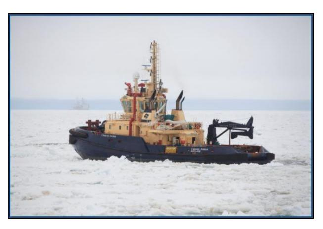
Operations in Prigorodnoye require support of the harbour tugs. Sakhalin Energy operates four purpose built ice class 1A tugs equipped with Aquamaster propulsion system (Z drive).
