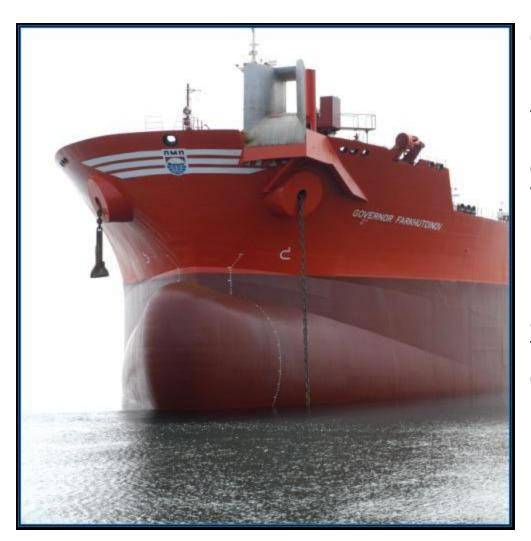
Oil tankers loading at Prigorodnoye during winter months are ice class 1C and fitted with the special bow loading arrangements designed by Pusnes to keep the loading hose clear of ice.
