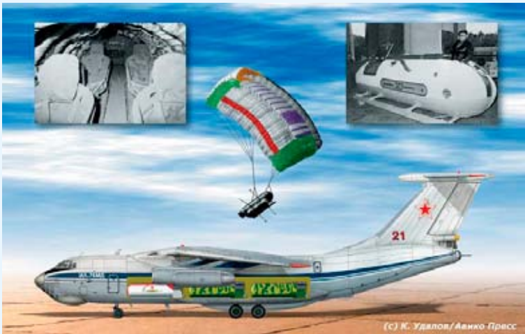
Figure A11 – Ganymede container-cabin concept for rapid deployment EER response (source: Central Marine Research and Design Institute)
