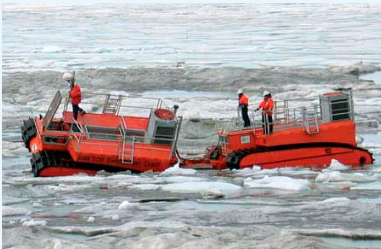
Figure A1 - ARKTOS evacuation craft undergoing pilot training in the US Beaufort Sea (source: ARKTOS Development Ltd.)
