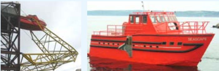
Figure A6 - Seascope deployment system and rescue craft (source: Gardin-Haag BV)
