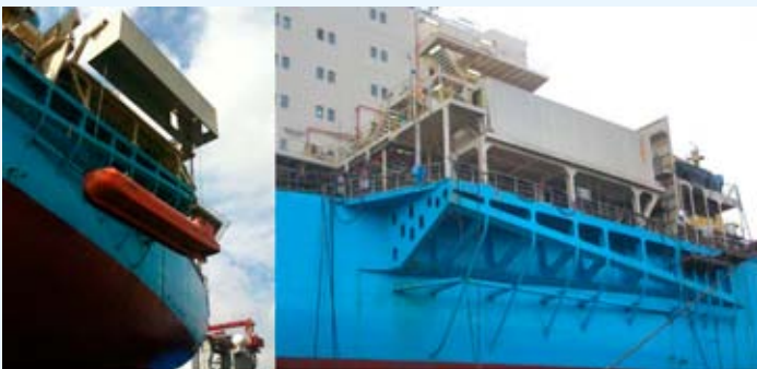
Figure A3 - A Boat-In-A-Box installation, in launched and stowed positions (source: Barr et al)
