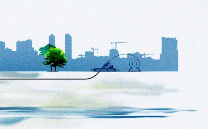
By transferring progress to the bit and replacing the drill string with coiled tubing, the Ultra No-Dig system can drive microtunnels in any desired direction for up to 30 kilometres.
