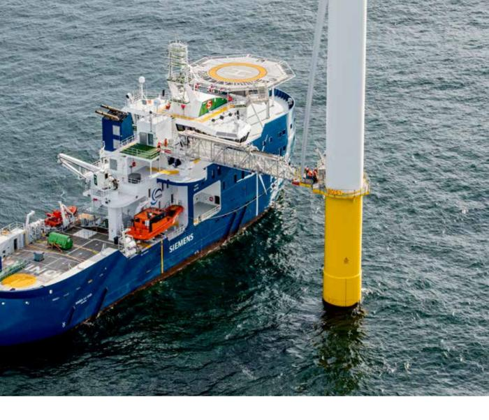
lift in an adjustable pedestal and across the gangway on electric trollies. That means technical personnel do not have to carry tools and equipment. Work on and maintenance of the turbines can be carried out without the need for cranes.
